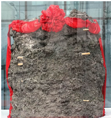
Figure 2: The largest single titanium sponge ever produced, at the 2011 world conference on titanium. Author photo.
