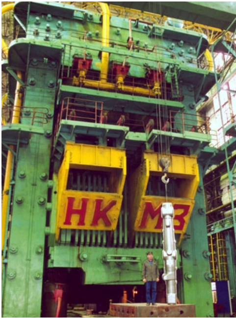
Figure 23: The 75,000 tonne (750 MN) press at VSMPO in Verkhanya Salda, Russia. The component is an 8-ton B-777 Ti-10-2-3 truck beam forging, with a man for scale.
