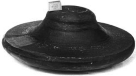
Figure 22: Photograph of a turbine disc forging, in IN718. Notice that the forging blank is much larger than the final disc shape - often > 90% of the material is machined away.
