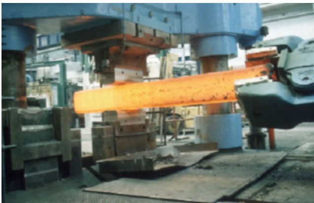
Figure 18: Photograph of a billet being open die forged (cogged).
