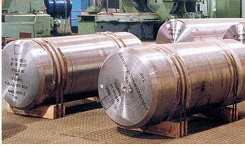
Figure 17: Rough machined VAR ingots on a factory floor, awaiting forging.
