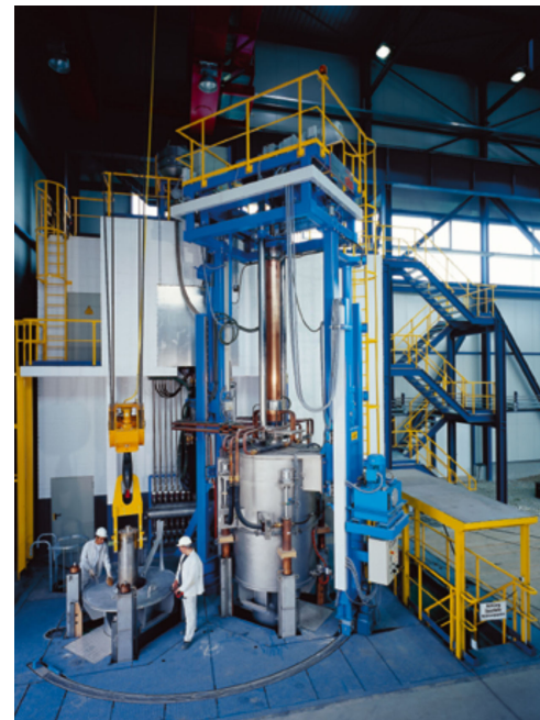
Figure 14: Photograph of the top of an ESR furnace.
