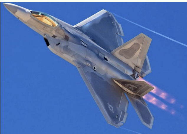
Figure 3: The F22 fighter aircraft, the airframe of which is 42% Ti, 24% polymer matrix composite (PMC), 24% aluminium alloy and 10% steels. At the beginning of manufacturing development a majority PMC share was planned.
